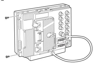
**3** Remove the two screws, and remove the main controls from the main unit. These two screws cannot be removed from the main controls themselves.
